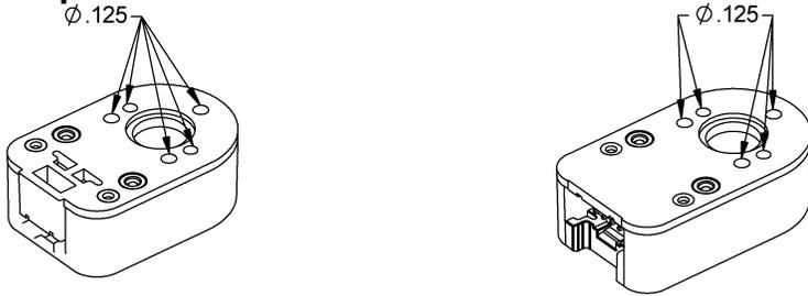
The 3-option makes all five of these hole diameters .125". The .438" diameter center hole can also mate with a motor boss.
