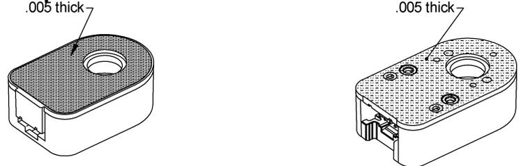
When mounting holes are not available, a pre-applied transfer adhesive (with peel-off backing) is available for "stick-on" mounting. Use the centering tool (sold separately) to slide the base into position. T-option specifies transfer adhesive on the standard mounting base.
