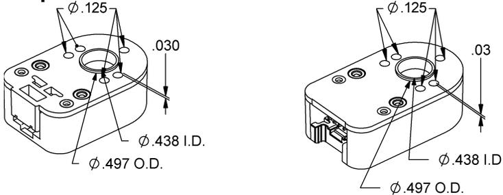
The A-option adds a .497" diameter alignment shoulder designed to slip into a .500" diameter recess in the mounting surface centered around the shaft.
