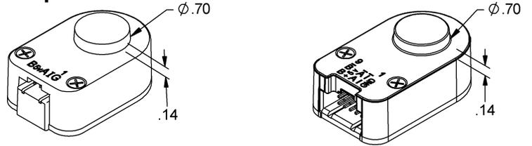
The E-option provides a cylindrical extension to the cover allowing for longer shafts of up to .750".
