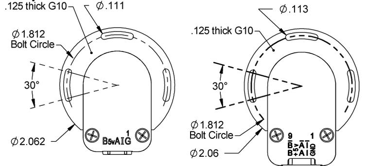
This adapter is an 1/8" thick fiberglass adapter which is pre-mounted to the base of the encoder. It allows the E5 to be rotated  $\pm 15^\circ$  while operating for index orientation. Use three 4-40 x 1/4" screws (sold separately). When installing the hub, with the 3 screws loose, rotate while operating to the desired index location and tighten. Note that this adds 1/8" to the required shaft length. **Please note:** Only available in polycarbonate versions (E5D and E5S).
