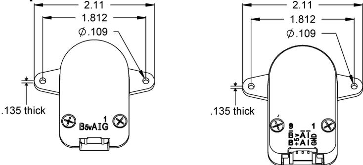
This option includes molded ears on the E5 base which enable it to be mounted to a 1.812" diameter bolt circle. The mounting holes are designed to fit 4-40 screws. Because the ears are molded to the E5 base this does not increase the thickness of the encoder and does not add to the required shaft length. This option will work with shaft lengths of .445" to .570"
